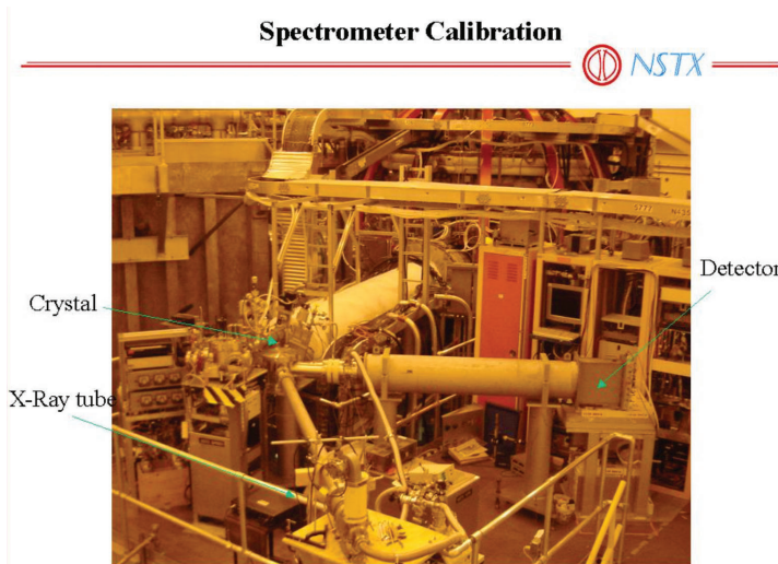
Figure 3. In situ calibration of the X-ray imaging crystal spectrometer at the National Spherical Torus Experiment (NSTX) in Princeton, NJ with use of an X-ray tube. The 10 cm diameter spherical crystal is housed at the point shown.
