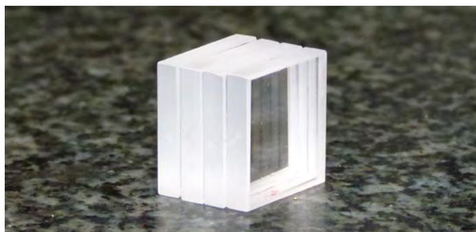
**Figure 2:** Contacted walk-off compensated  $\beta\text{-BBO}$  assembly produced at Inrad Optics, Inc.
